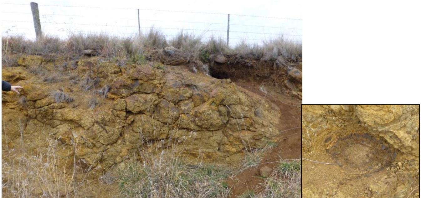
Figure 4 (left). As the basalt corestones weather they are replaced by secondary clay minerals, typically smectite and kaolinite clays, with yellow brown or red brown coloration due to minor amounts of hematite and/or goethite, Ravensworth TSR. Figure 5 (right). Concentric weathering of a basaltic corestone shows the 'onion skin' texture that results from hydrolysis of rock to form secondary clays and sesquioxides, Ravensworth TSR.
