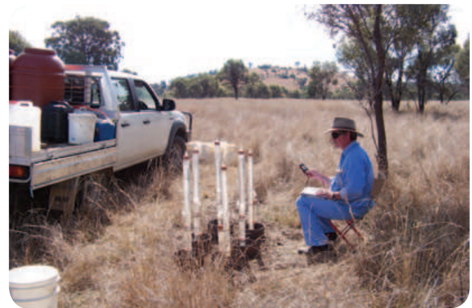
Measuring water filtration rates into the soil profile tells a story of soil structure, stability and productivity.
