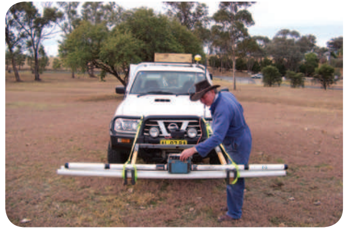
Measuring soil salinity trends using electro-magnetic induction device: Inverell NSW.
